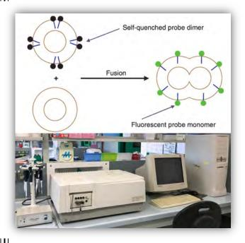
The aim of this training is to monitor, in real-time, the fusion between membranes using a fluorimetric method for assaying membrane fusion exploit processes in a cell-free model system that reflects the step of exocytosis. Specifically, final isolated vesicles are labeled with a lipidfluorescent soluble probe (octadecylrhodamine) self-R18). at concentration quenching and. as a consequence of fusion with unlabelled membrane, lipid probe dilution occurs,
