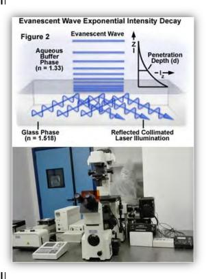
TIRFM is a well-established method to study water and solute permeabilities and cell volume regulation in cells of arbitrary shape and size. Adherent cells labeled with an aqueous-phase dye, are rapidly exposed to an osmotic gradient and the time course of fluorescence signal is detected.
